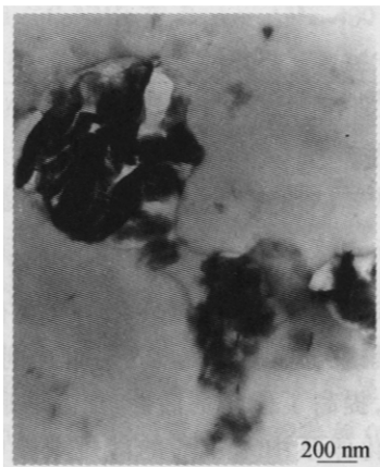
Fig. 7 TEM photograph of sPS/MTN (melt-mixing)
